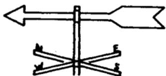
5. This is an instrument which gives the direction from which the wind is blowing. In the United States, the north wind is a cold wind and the south wind is a warm wind.
