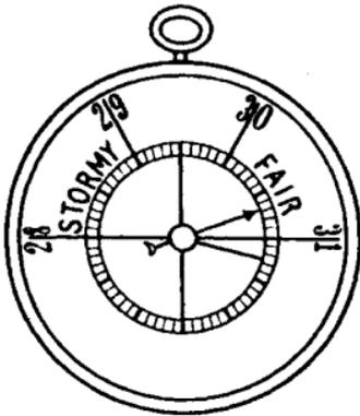
2. This is an instrument for measuring the weight of the air. Galileo was the first person who made the discovery that air has weight. Warm air goes up because it has less weight than cold air.
